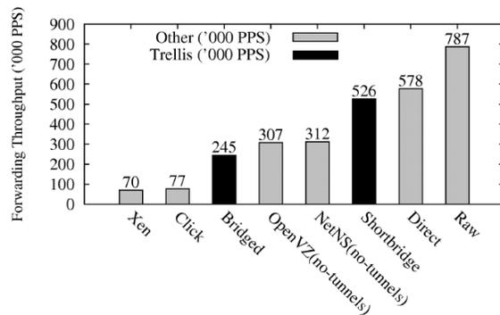
Figure 4: Peak forwarding performance in pps with 64byte packets [BHA2008]
