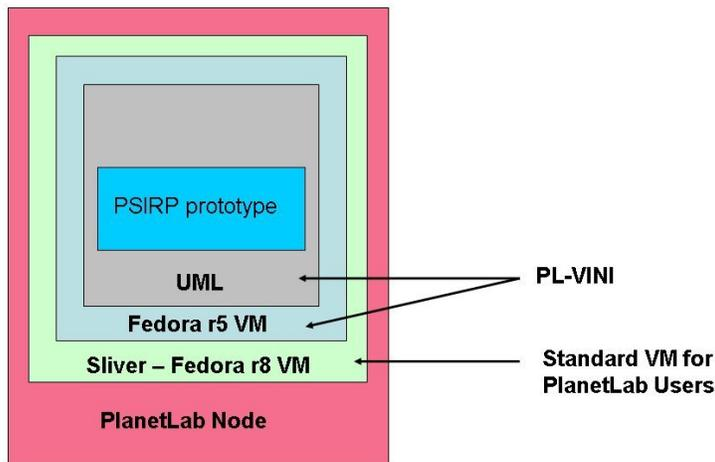
Figure 7: PSIRP prototype virtual machine layering on a PlanetLab node
