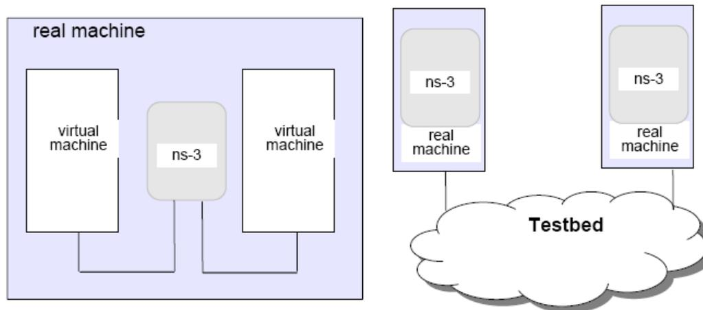
**Figure 6: ns-3 interconnecting virtual machines, and testbeds interconnecting ns-3 stacks [NS32009a]**
