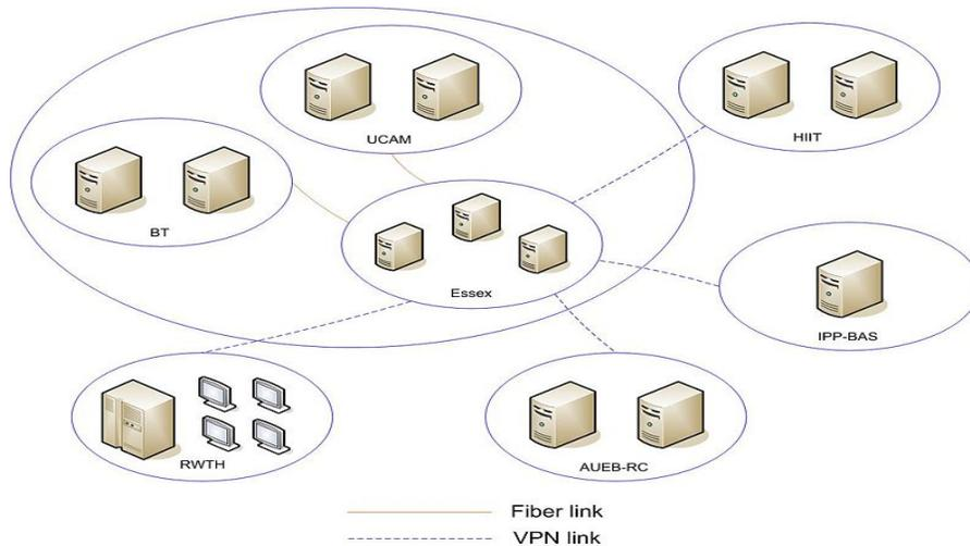
**Fig. 1 – PSIRP test bed setup**
